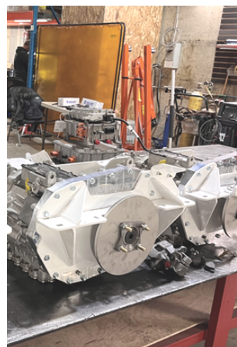
INTEGRATION OF ELECTRIC ENGINE INTO THE EXISTING BAGGAGE TRACTOR
